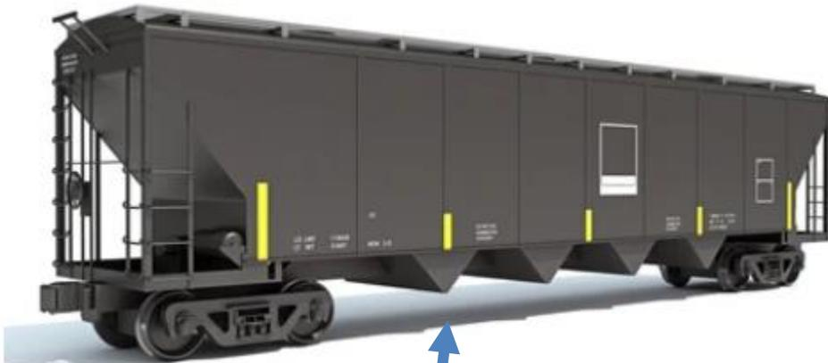
Normal “hopper” style rail cars SHOULD NOT be used as sulfide particles (“fines”) will fall through the hopper doors on the bottom
