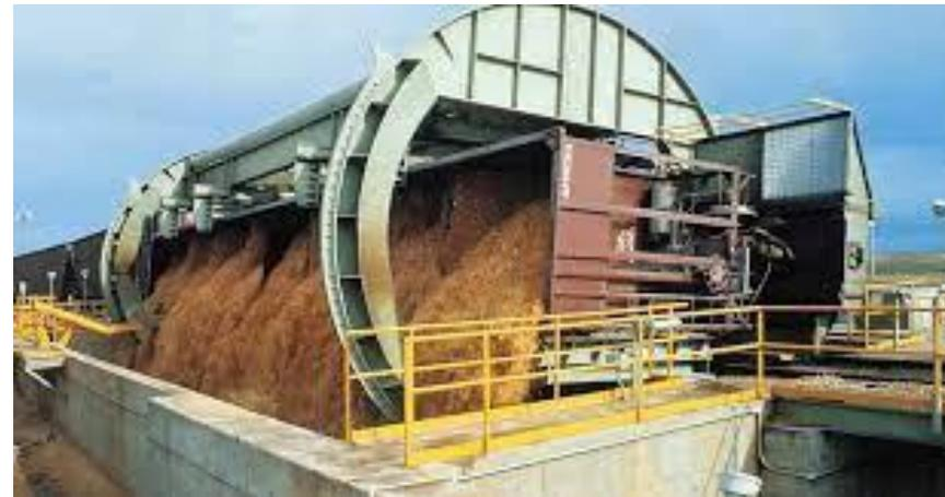
Gondola cars may work BUT many gondola cars still have openings in the bottom that can leak materials. These have to be flipped upside down to empty since there is no bottom hatch. This will require a 'rotary car dumper' in North Dakota.
